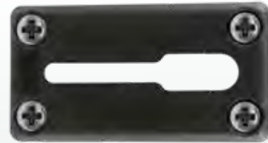
439 GEAR HEAD TRACK ADAPTER Mount track accessories to your inflatable watercraft's pre-installed 341 mounts. Fasten track to 341 mount with supplied 1/4-20 x .5" stainless steel bolts. Slide and lock our 438 gear head Adapter or ball mount onto the track.
